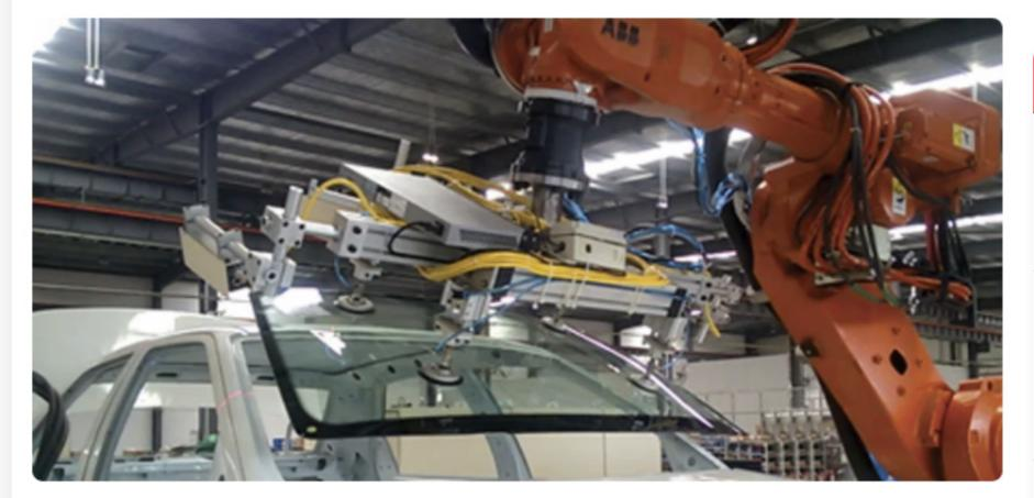
Automobile manufacturers are employing vision-equipped robotic insertion systems to ensure the correct placement of vehicle closures such as windshields, hoods, trunk lids and doors. When deployed on the production line, these systems are used to pick up and accurately place everything from the roof panels to windshields and load them onto the car body's framework. These part loading or insertion applications are a real challenge for vision system designers due to several factors.
