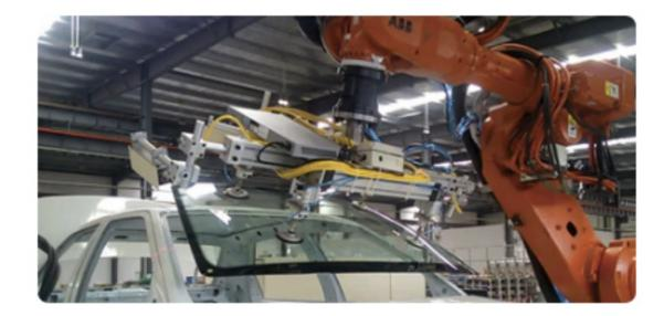
Bluewrist engineers utilized the built-in edge tool of four Gocator 2300 series 3D smart sensors on the robot end effector to monitor the location of 4 critical points on the windshield aperture.
