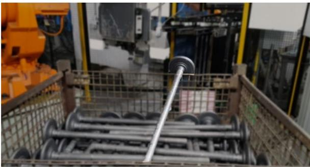
Reliable detection of misplaced parts in bin and collision check
