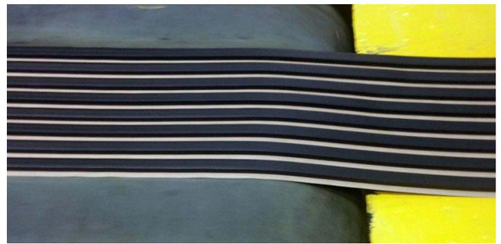
Actual weather sealant tape produced in upstream process
