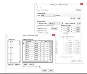
EzRG advanced robot guidance software provides a wide range of robot guidance and user-frame calculation strategies including Best-fit of Measurement, 3-2-1 Fixturing, and a
