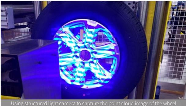
Using structured light camera to capture the point cloud image of the wheel
