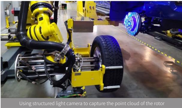
Using structured light camera to capture the point cloud of the rotor
