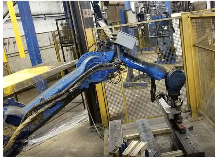
Material Handling Robot Picking Up Part from Stack
