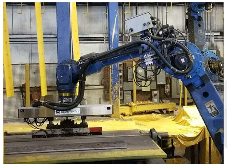
Picked Part is Transferred to Scanning Table
