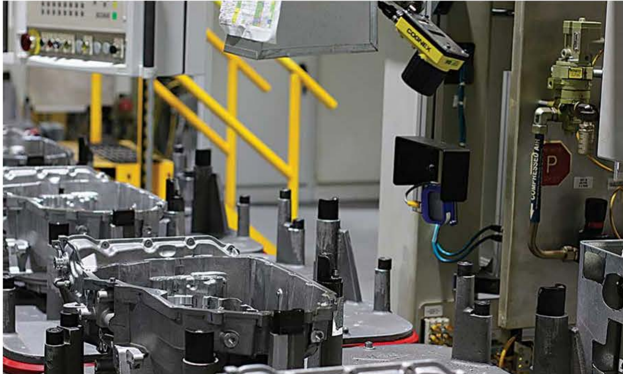
Machine vision technology is used by automakers and suppliers for a variety of applications, including error-proofing and inline inspection. Photo courtesy Ford Motor Co.
